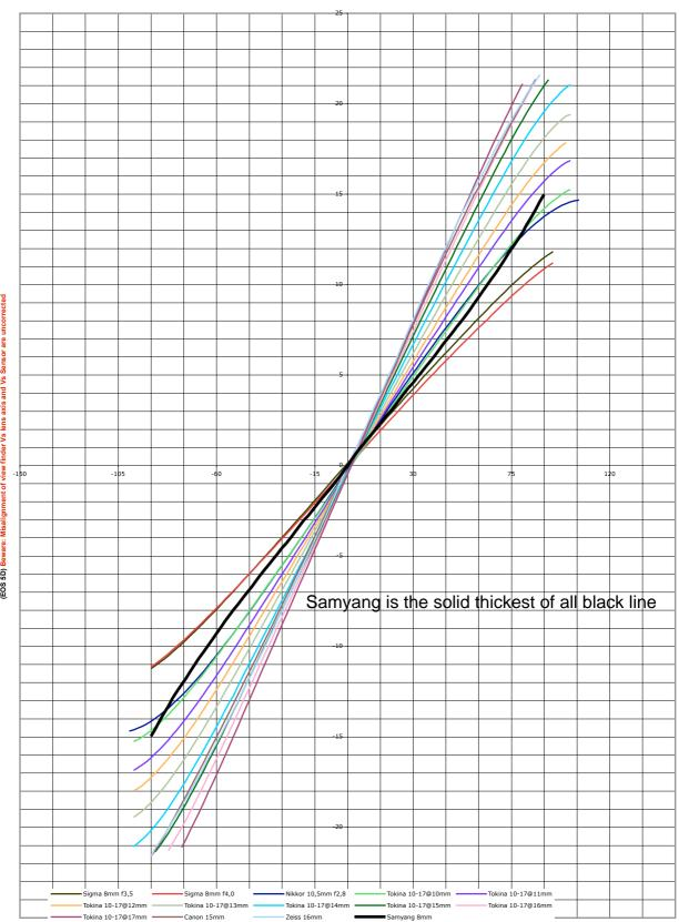
Distance from center ( mm) mes ured on the captured image of a cylindrical target (EOS 5D) Beware: Misalignment of view finder Vs lens axis and Vs Sensor are uncorrected
